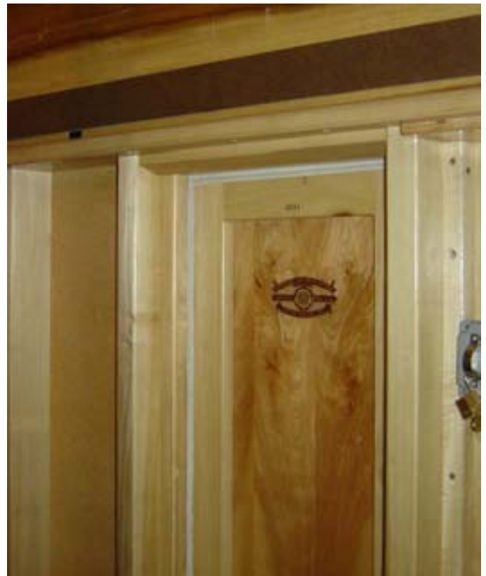
This is the Airbox door. The door is gasketed all around, to ensure air-tight seal, and bears the famous Austin Universal Airchest logo, indicating a true Austin Airchest System as designed by John T. Austin, and built by the company ever since.
