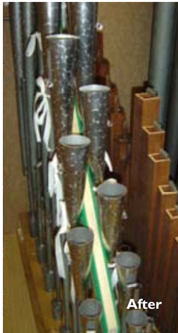
On the left, we see the old Oboe & Bassoon. The bells, made of traditional common metal were all but destroyed from years of tuning, and... gravity! They were used as patterns for the new bells, made of spotted metal.
