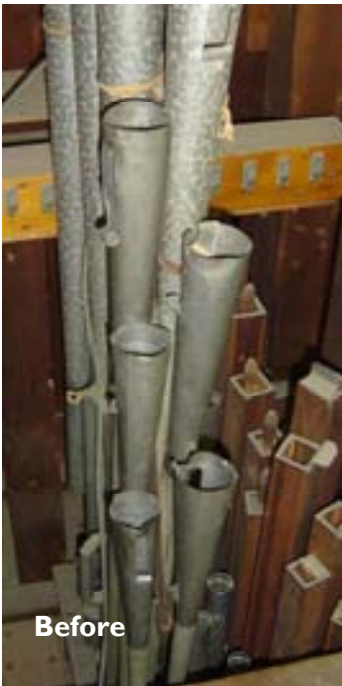
On the left, we see the old Oboe & Bassoon. The bells, made of traditional common metal were all but destroyed from years of tuning, and... gravity! They were used as patterns for the new bells, made of spotted metal.
