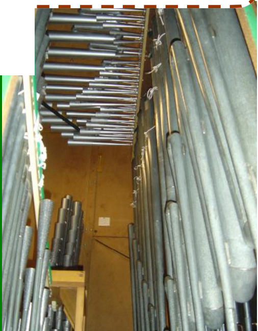
A view inside the Swell Organ. The Tuba (en chamade) above, the new 8' Hautbois and Trompette on left and the 16' Trompette on right.
